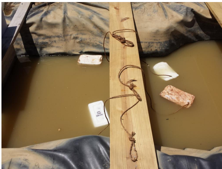
Figure 2.4: Photograph of four 703d type Floc Logs suspended in the turbidity test channel. Photo taken by author.
