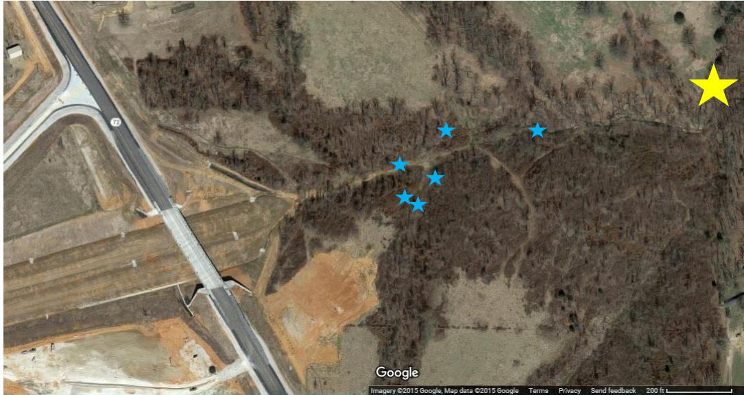
Figure 2.3: A picture taken from Google Maps®. The yellow-colored star located on the right side of the picture shows the approximate location where sampling took place. The blue-colored stars show the approximate location of the placement of each 703d#3 Floc Log for the second field test.
