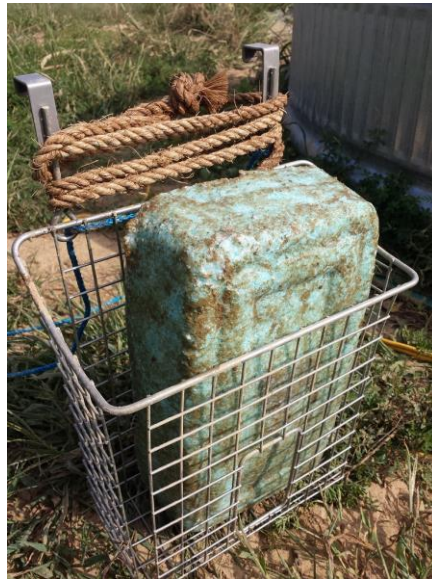
Figure 2.6: A single 703d#3 Floc Log placed inside of a cage container used for the eight consecutive basin-scale jar tests. Photo taken by author.
